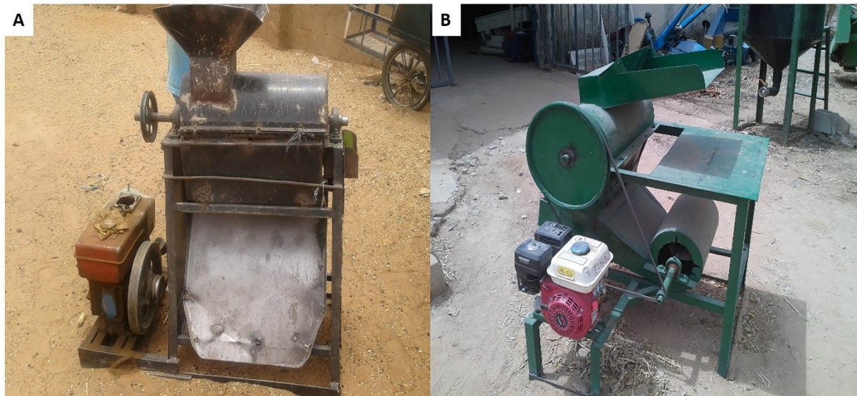
Figure 4: Locally made groundnut sheller (A) and new groundnut sheller after modification (B)
